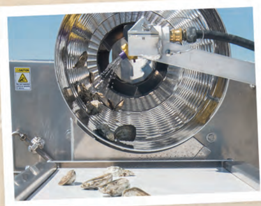
Oyster Tumbler Sort, wash and size oysters for market or further grow-out.
