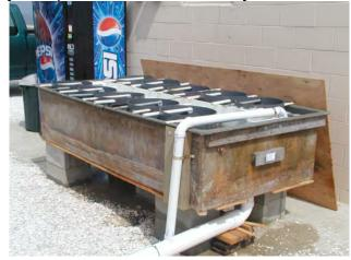
allow for good water flow. A hole large enough for a pipe is drilled near the top of the silo, and another hole is drilled at the same level through a center trough or the tank's side to establish the water level in the silo. The outflow
